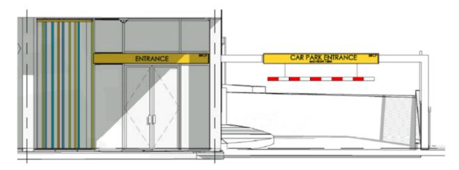
The new entrance doors with associated metal-framed glazed screens and vertical fin detail would create a simpler and more contemporary appearance than the existing. New concrete-sett paving along the undercroft area will also create a more consistent and improved appearance at the site frontage. Elsewhere the proposed white louvre infills to the existing stairwell windows are designed to deflect rain and address an existing maintenance issue.
